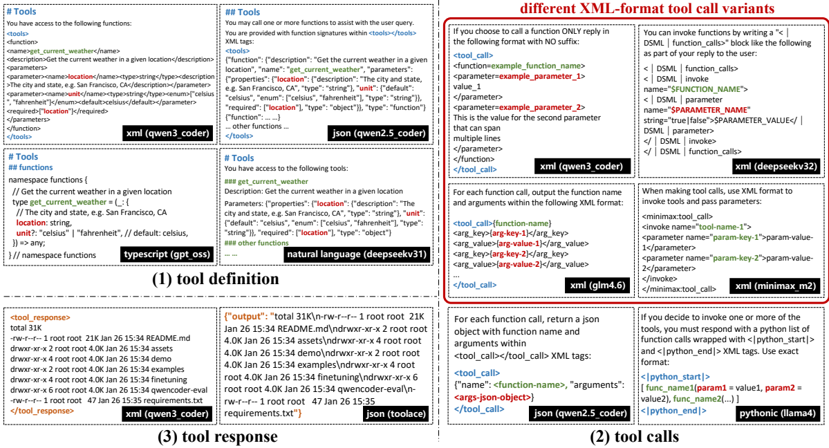
Figure 5: Different tool chat templates, split by tool definition, tool calls, and tool response.
